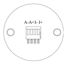
If the axle is kitted out for a plug ( LUMBERG), connectors are marked as following :
